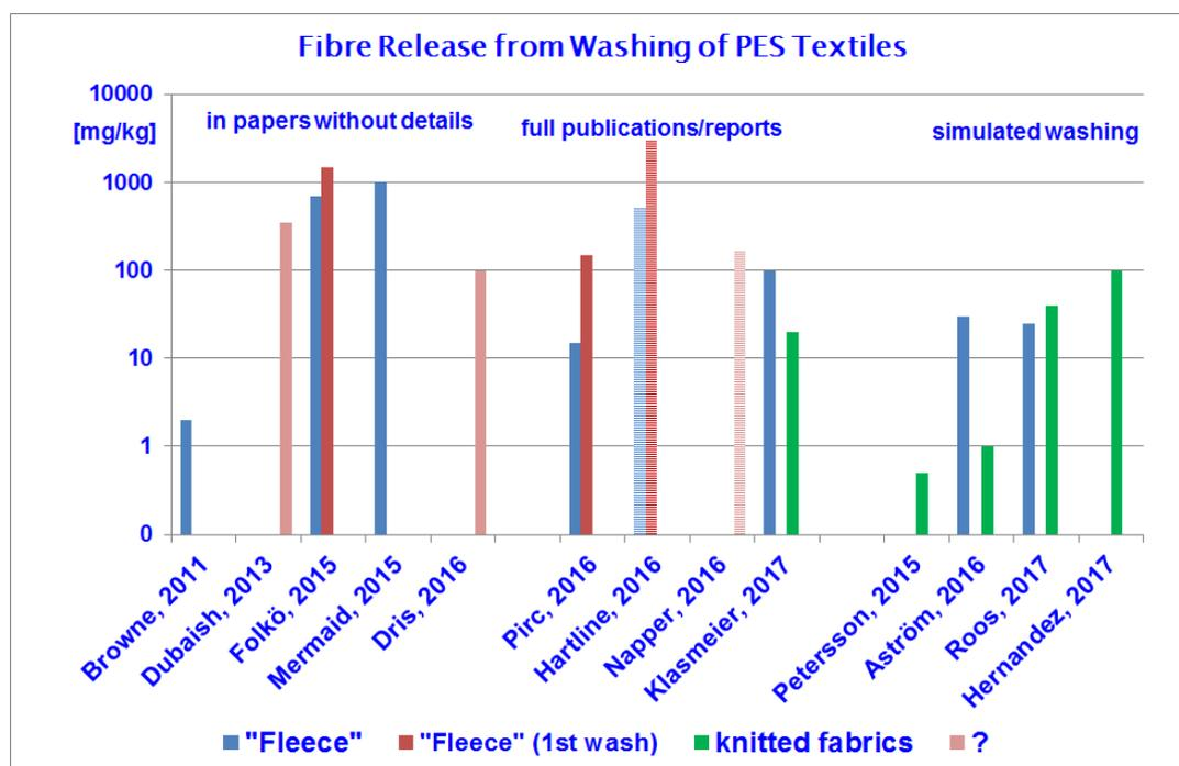
Fig. 1: Reported fibre releases from washing of PES textile products as mass ratios [mg per kg product]; in a logarithmic scale; explanations, see fig. 2 and 3, tables 1 – 3.
